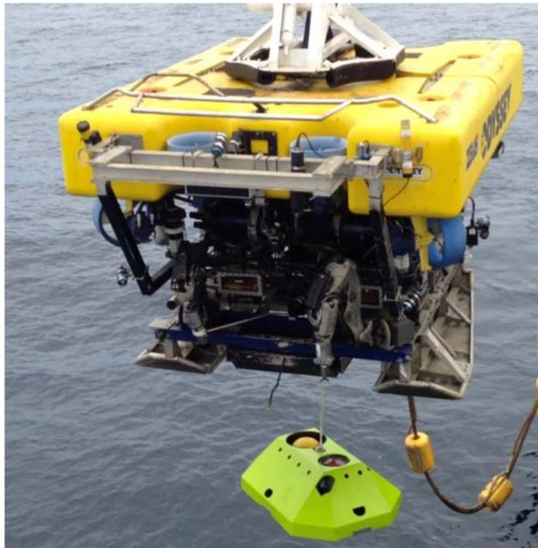
**ROV being lowered into the water with equipment to test water column currents and turbidity
